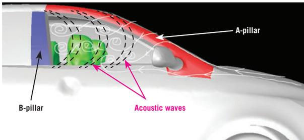
▲ Wind buffeting can intensify due to flow-acoustic feedback.
