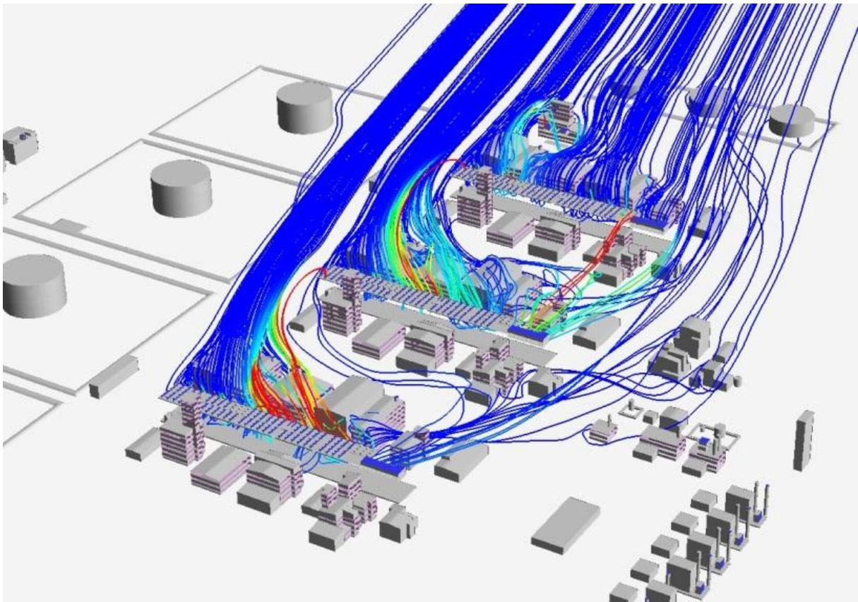
Image 2 - Pathlines tracked to the air cooler intakes coloured by temperature.
