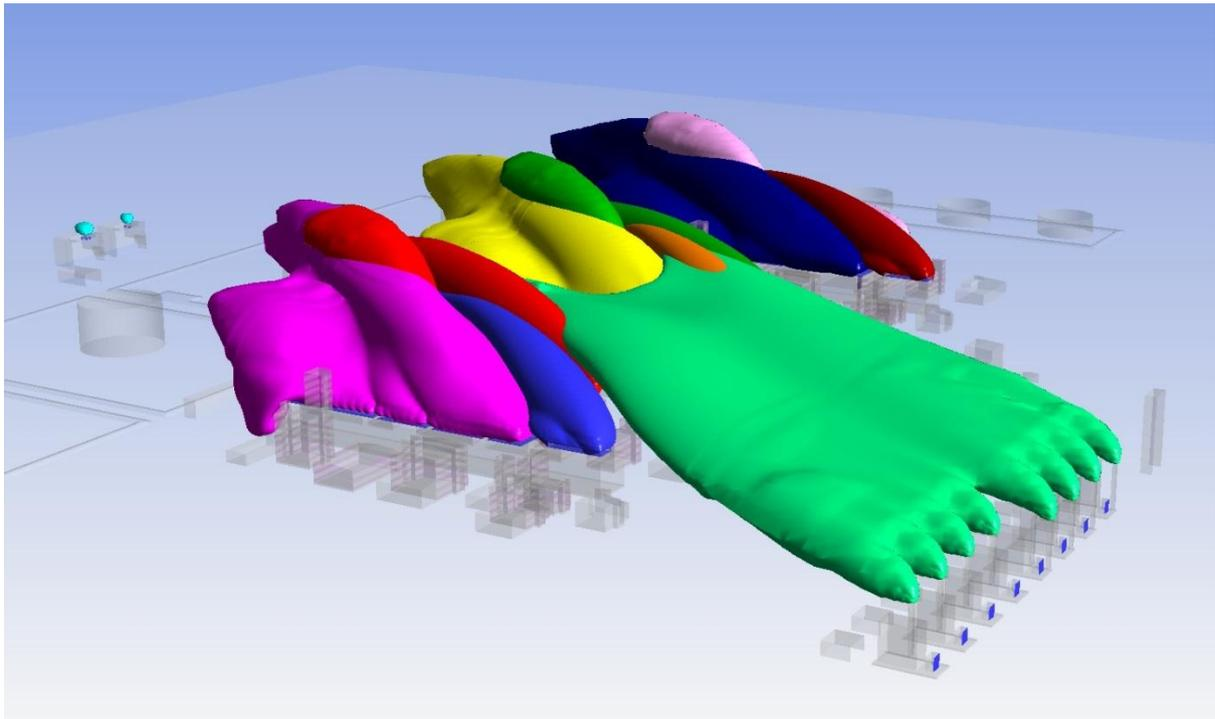
Image 1 - Hot air plume over the simulated Yamal LNG site coloured by the originating unit for the plumes.
