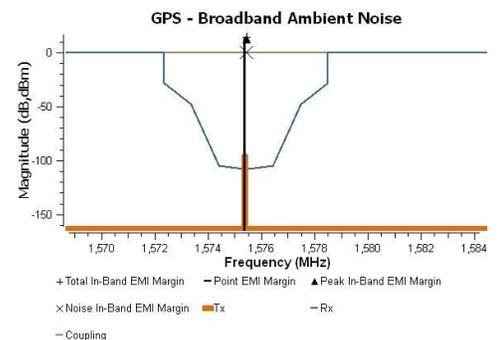
Detailed results plot displaying the interference in the GPS Rx due to the 25th harmonic of a 63.015 MHz oscillator.
