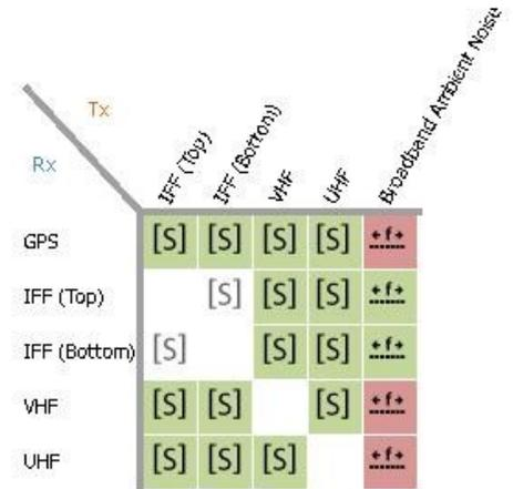
Threat matrix for Predator RF Systems with broadband ambient noise modeled. The green indicates no interference and the red indicates interference is likely.
