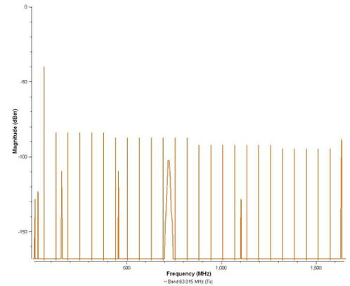
Measured broadband ambient noise spectrum resulting from electronic systems in the Predator fuselage
