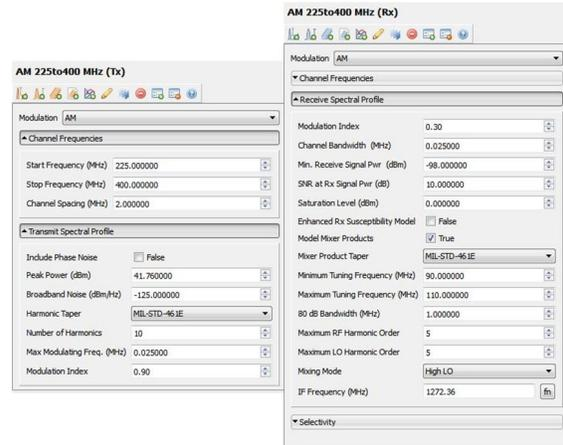
Sample transmitter and receiver properties showing the UHF Voice radio bands.
