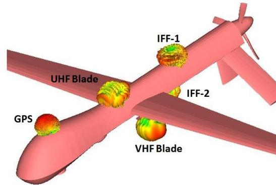
A Predator UAV with multiple RF Systems located at various points along the fuselage
