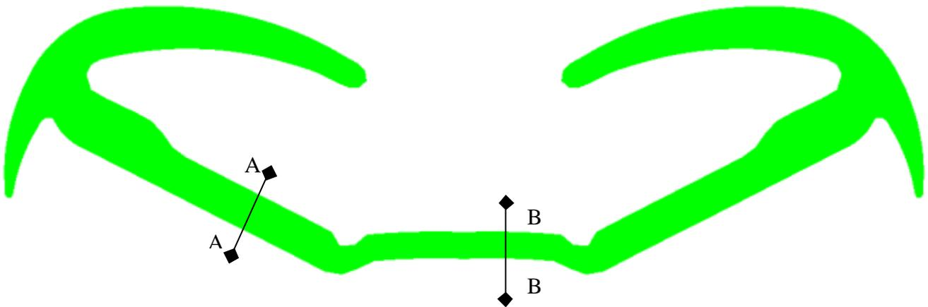
Figure 1 Targetted automotive profile. Comparison between the desired profile and the actual one is done along the section AA and BB
