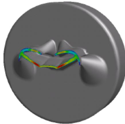
Figure 3.- Contour lines of the velocity magnitude across the die lip. A die land of 3 mm together with converging sections modify the velocity profile
