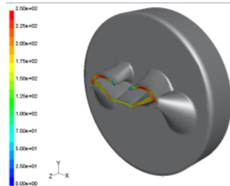
Figure 5 – Contour lines of the velocity magnitude across the die lip for the fully balanced die. The variation of the maximum velocity (in red) is much smaller than in Figure 2
