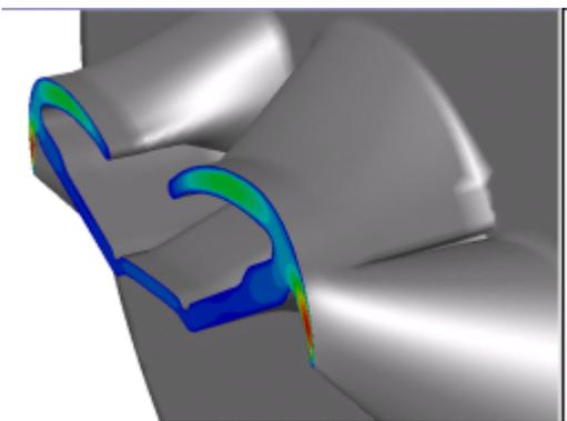
Figure 4.-Contour lines of the velocity magnitude. The die land has been removed close to section 5 inducing a too large local velocity .
