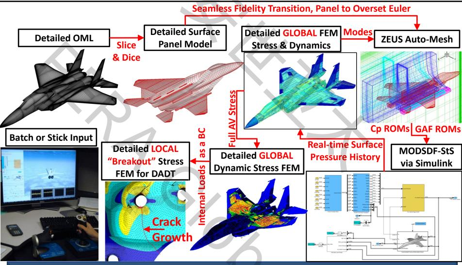
Detailed Mission-Vehicle-Pilot-Specific Dynamic Stress Histories for Fatigue, DADT & Fleet Management Purposes, all via Real-time Euler-based Simulation
